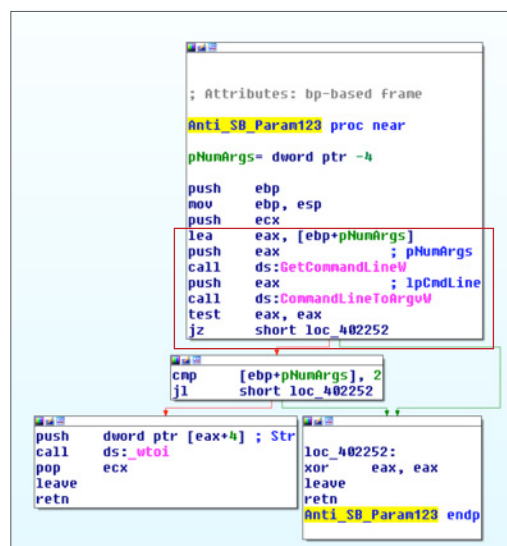
Figure 18: In this example, the command-line parameter "123" is passed by the infection vector, a JavaScript file. Then, the command-line parameter is read by the Windows API GetCommandLine and CommandLineToArgvW . (Hash: 0fed77b29961c0207bb4b7b033ca3fd4)
